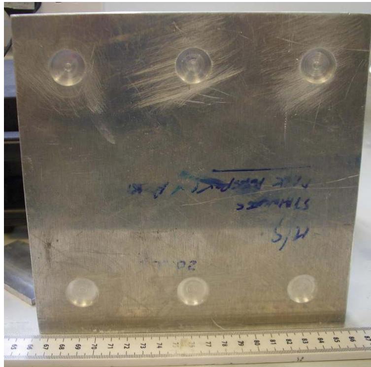
Fig 1. Aluminium test sample with 20mm \varnothing back-drilled hole defects at depths from 0.5mm to 3mm (0.5mm to 1.5mm top left to right, 2.0mm to 3.0mm bottom left to right)
